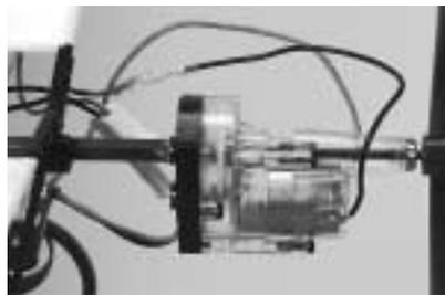
The Speed 280-size motor and 5.6:1 gearbox are enclosed in a clear plastic housing and slip easily onto the motor stick. The stick itself is carbon fiber, as are the rest of the structural elements.
