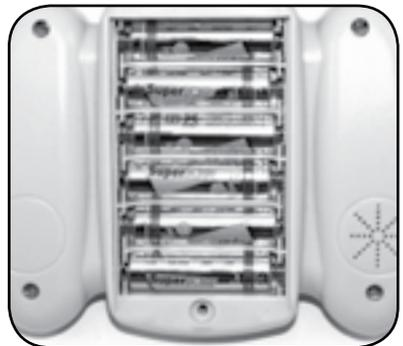
**IMPORTANT!** *If the transmitter batteries are not installed according to proper polarity, the transmitter will not function and electrical damage may occur.*
